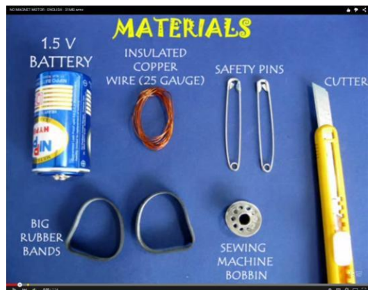
FIGURE 2. Materials needed to make a magnetic motor powered by electromagnet [11].
