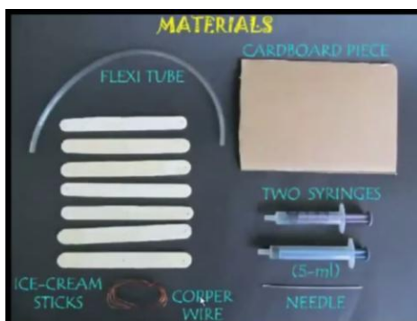
FIGURE 1. Materials required for demonstration of a hydraulic Jack [Reference 10].
